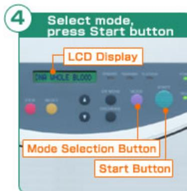
Figure 2. Method selection and start of QuickGene-810
